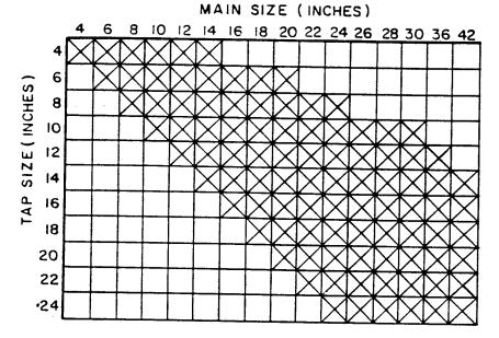
Any Thrust Reaction Block Requirements For Water Main And Tap Size Combinations Other Than Those Shown Above Will Require Special Design Approval By The CITY OF CRIPPLE CREEK DEPARTMENT OF PUBLIC WORKS.
